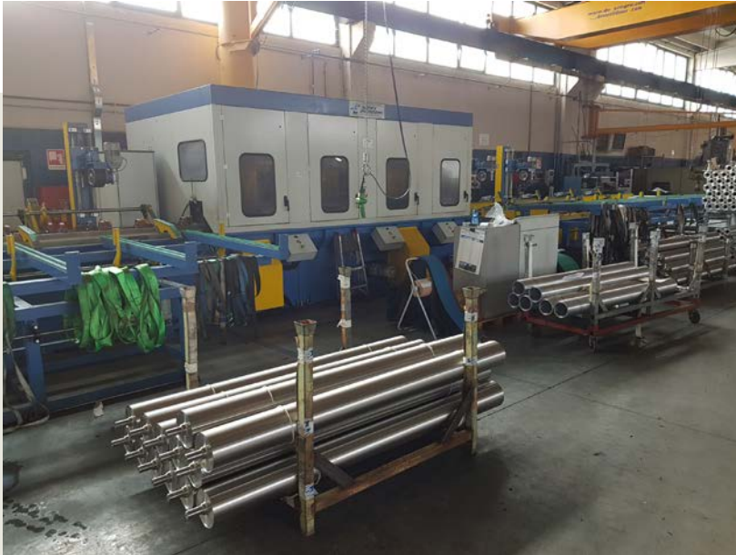
Brushing machine centreless up to \varnothing 220 and with centre up to \varnothing 1000 .
